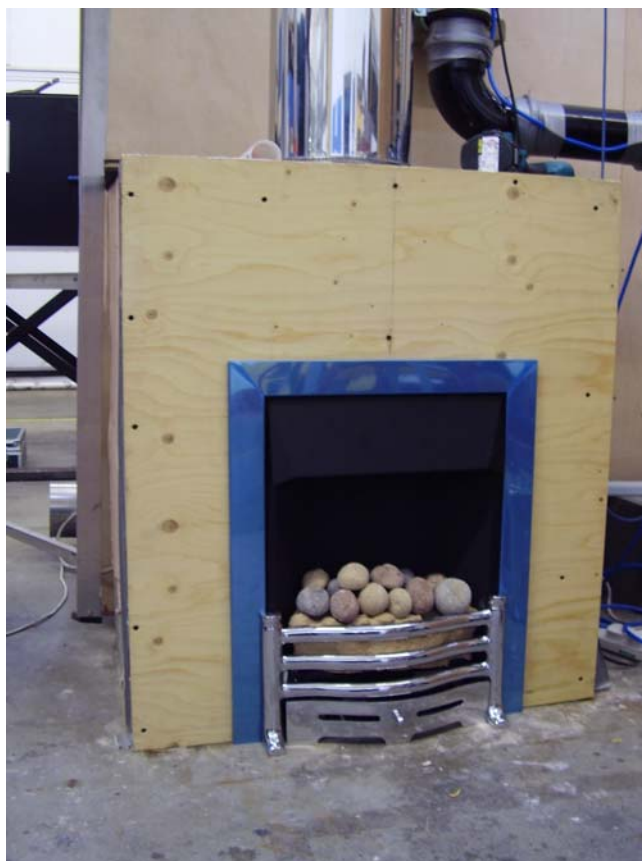
Figure 5 Installation of ILFE Fire
