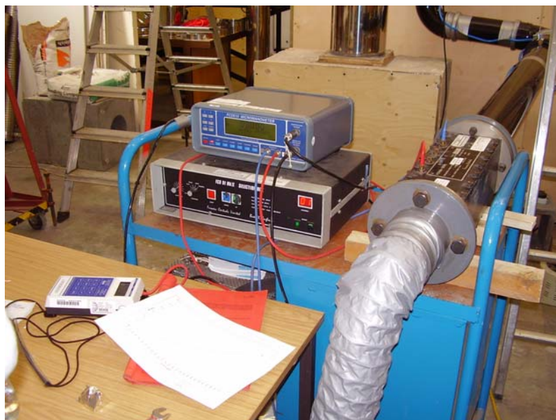
Figure 3 Air Flow measuring system and instrumentation
